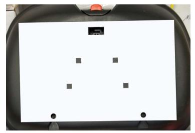
Clean the surface of Givi box (alcohol pad or similar recommended). See the **suggested** guide above for placement (optimal placement of bumpers differs by top box. or most secure fit, apply where maximum contact occurs between rack and top box). Bumpers can be applied on rack or top box.
