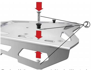
Assemble the posts as shown, in this order: M6-post-rack-washer-nylock nut. No thread locker is necessary.
